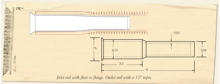
An integral fin tube typically has a plain end of 2" long then a transition to the ID under the fins. Ferrules are designed to compensate for the two different ID's. The inlet end has
